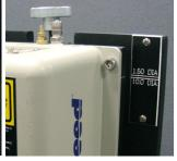
The LaserSpeed gauge is mounted to a heavy-duty sliding rail. A rotating knob enables you to adjust the gauge height, while the position indicator lets you precisely set the measurement distance for the specific product size.
