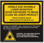
The following safety features required to comply with the Bureau of Radiological Health Class IIIB laser requirements are included:
