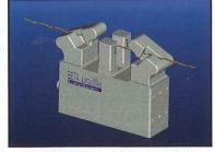
ments with the highest precision to within 1 mil. Providing high-data rate capabilities, LayScan precisely determines the variations in lay length within each lay, and systematic lay variations that are typically caused by twinning and cabling operations can be readily observed and measured, the release said. It added that a data acquisition system effectively collects and processes the lay length data and reports the measurement results.
